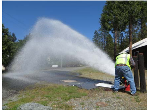
Hydrant testing using the "diffuser."
